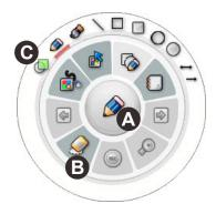
Floating toolbar comprises 3 sections A, B, C and each section is connected hierarchically.
